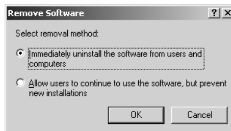
FIGURE 12.30 Removing the package immediately
